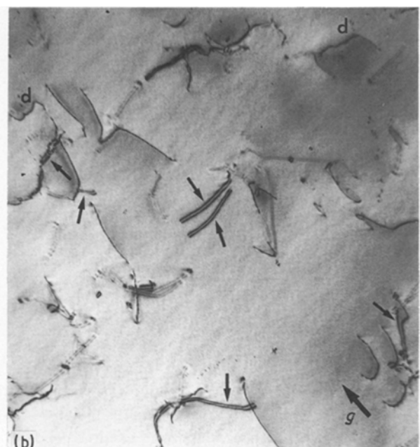
Figure 14 Pair of micrographs using opposite sign g vector to illustrate the large number of dipoles (arrowed). Annealed 120s at 500°C.
