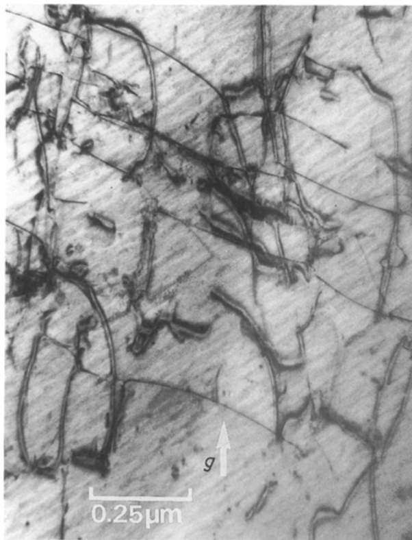
Figure 8 Superdislocations remaining within unrecrystallized part after annealing 30 s at 440 °C.
