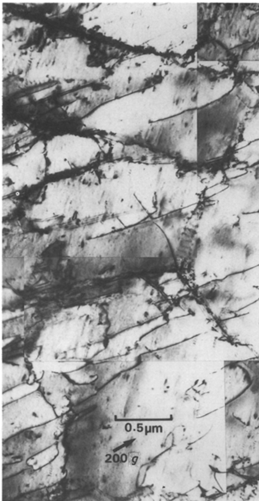
Figure 12 Partially recovered dislocation structure within the unrecrystallized parts after annealing 10s at 500°C to recrystallized 5%.
